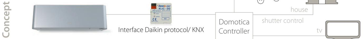
Connect Sky Air / VRV indoor units to KNX interface for BMS integration
